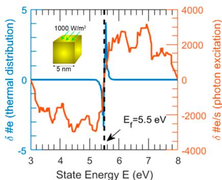
**Figure 2.** Hot electron generation rate under 532 nm monochromatic irradiation at a power density of 1000 W/m<sup>2</sup> compared with the thermal distribution of electrons in a 5 nm Au cube at 300 K.
